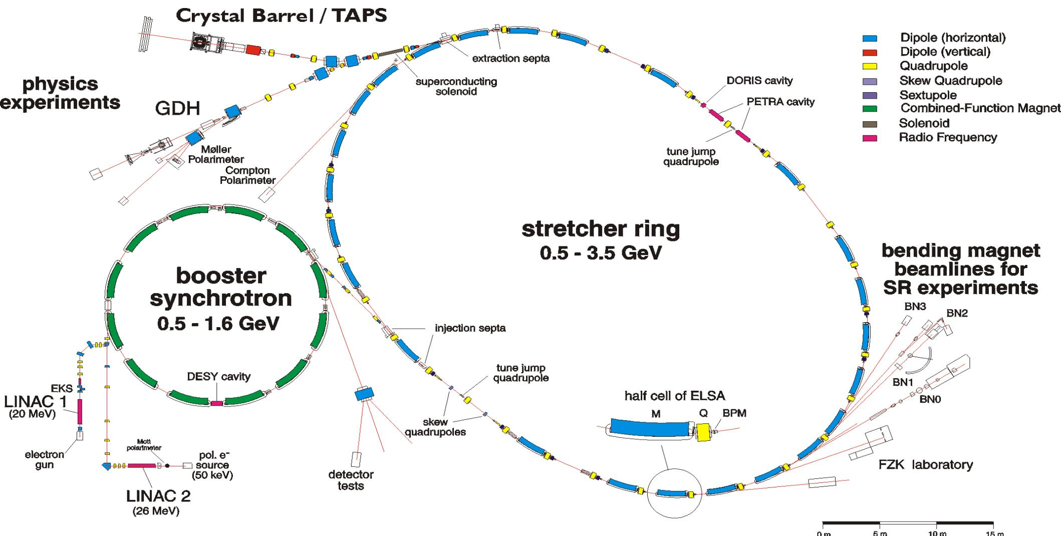
quasi-monochromatic photon beam via bremsstrahlungs tagging
