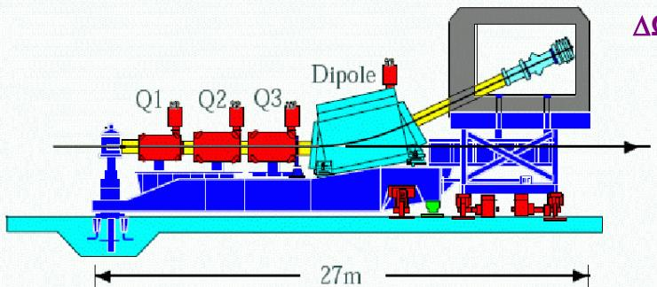
Short Orbit Spectrometer:  $P_{max} = 1.74 \text{ GeV}/c$   $\Delta P = \pm 20\%$
